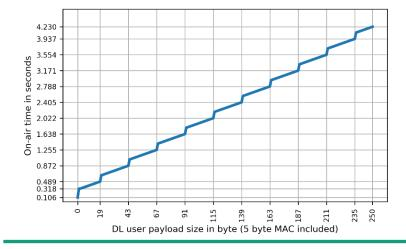
**Downlink transmission rate** for base station duty cycle of 10%
